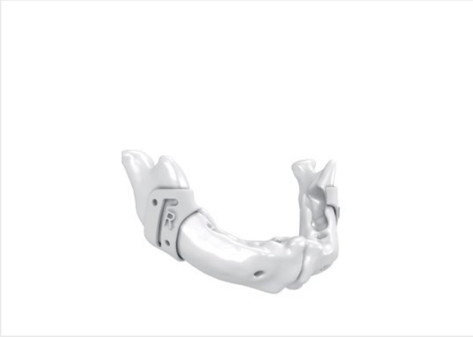
Unilateral distraction of the mandible Patient-specific marking guide for Zurich II Distractor
