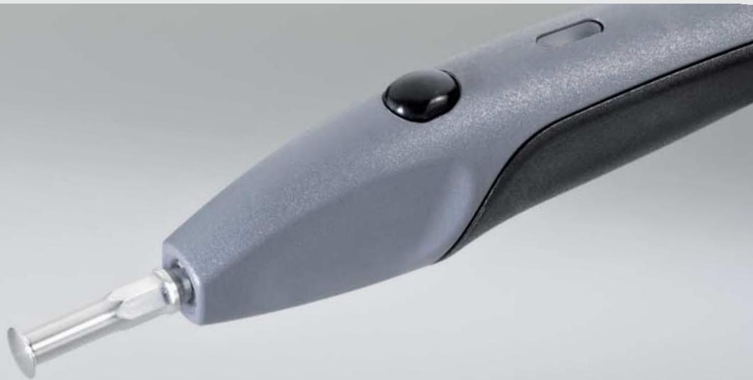
The ultrasonic unit of the SonicWeld Rx® system converts electric energy into mechanical vibrations (ultrasound).
